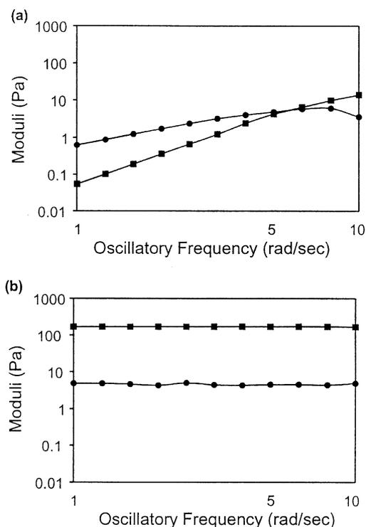
Fig. 2. Primary data for gel formation of 1 wt% KFE12 equilibrated with (a) 0.1 mM NaCl and (b) 1.0 mM NaCl. The storage modulus (squares),  $G'$ , and loss modulus (circles),  $G''$ , are plotted against oscillatory frequency on log–log scales.
