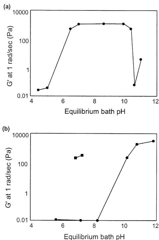
Fig. 6. Rheology results for addition of NaOH. Data for  $G'$  at 1 rad/s for (a) KFE12 and (b) KFQ12 equilibrated in various concentrations of NaOH. The pH of the bath at equilibrium was measured after each experiment and is plotted on the x-axis. The squares in (b) represent experiments on KFQ12 to which NaOH and 150 mM NaCl were added; the equilibrium bath pH was measured after the experiment.
